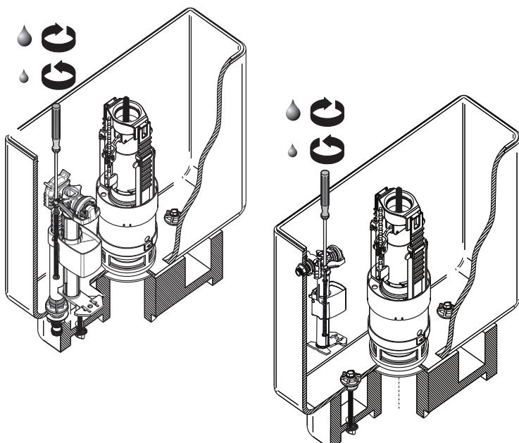
MANUTENÇÃO DA VÁLVULA OUTLET VALVE MAINTENANCE ENTRETIEN DU SOUPAPE RÉGLÉE MANTENIMIENTO DEL DESCARGADOR
